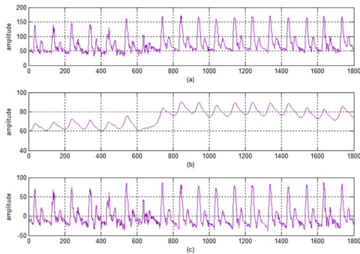
Fig. 3 Removal of baseline drift of pulse signal. (a) Original signal. (b) Trend line. (c) The signal of removing baseline drift.
