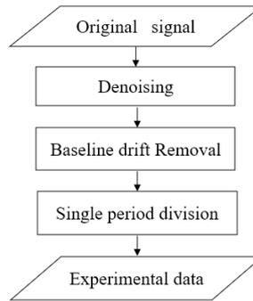
Fig. 2: Flow chart of pulse signal preprocessing.
